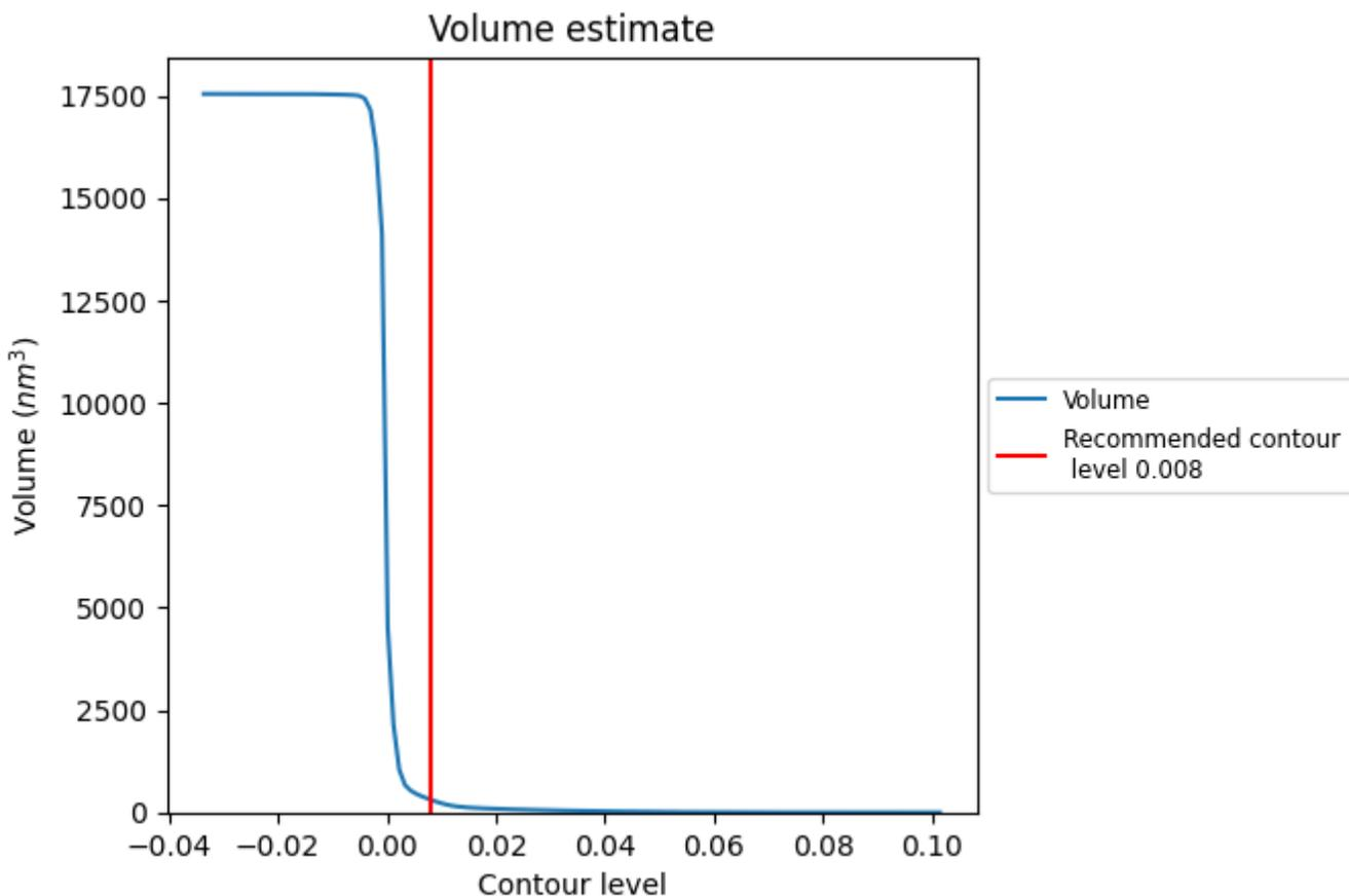
The volume at the recommended contour level is 311  $\text{nm}^3$ ; this corresponds to an approximate mass of 281 kDa.
