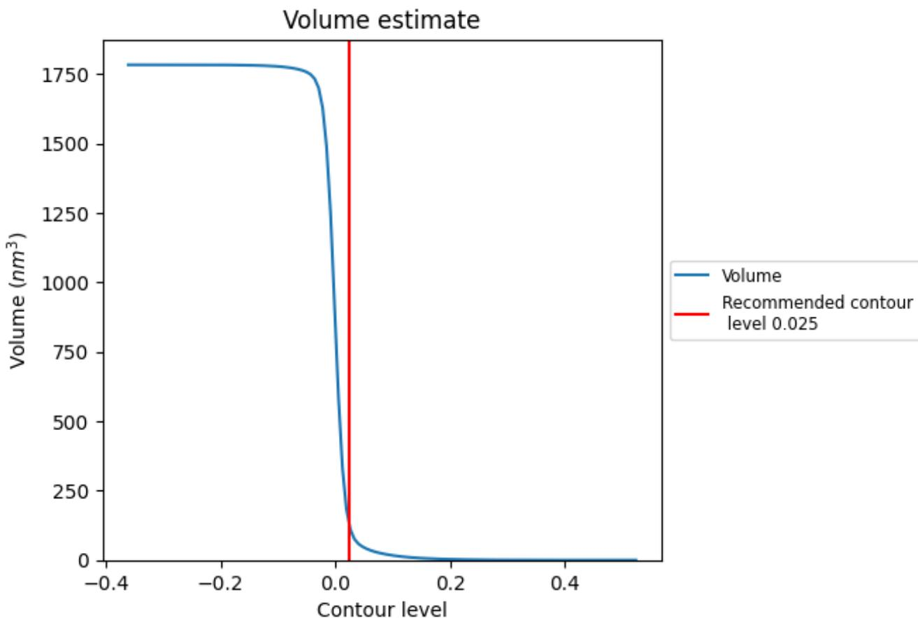
The volume at the recommended contour level is  $120 \text{ nm}^3$ ; this corresponds to an approximate mass of 108 kDa.
