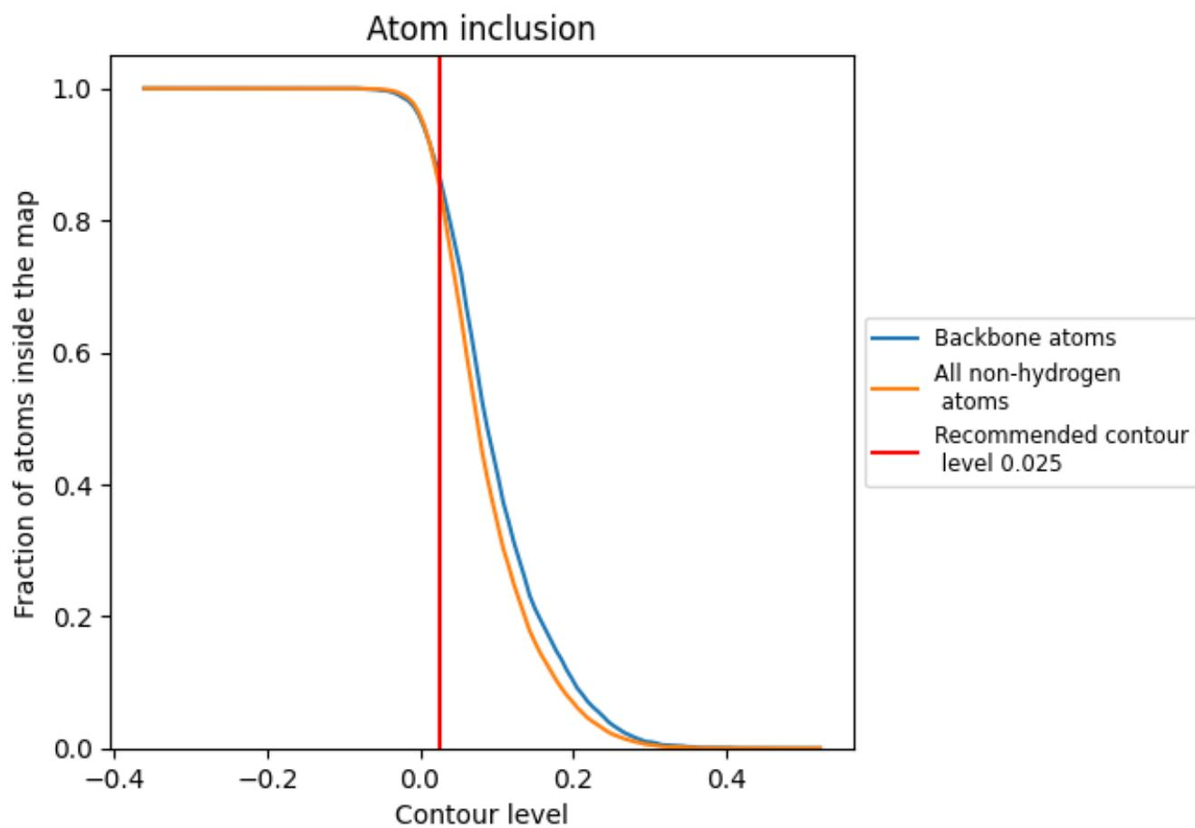
At the recommended contour level, 87% of all backbone atoms, 85% of all non-hydrogen atoms, are inside the map.
