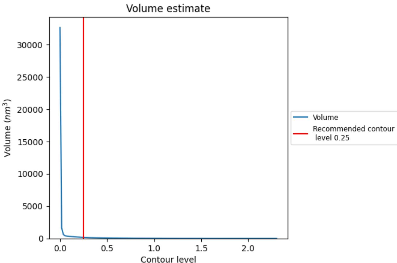
The volume at the recommended contour level is 166  $\text{nm}^3$ ; this corresponds to an approximate mass of 150 kDa.
