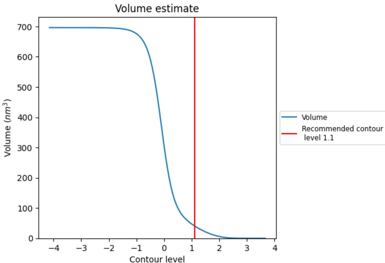
The volume at the recommended contour level is 41 nm<sup>3</sup>; this corresponds to an approximate mass of 37 kDa.
