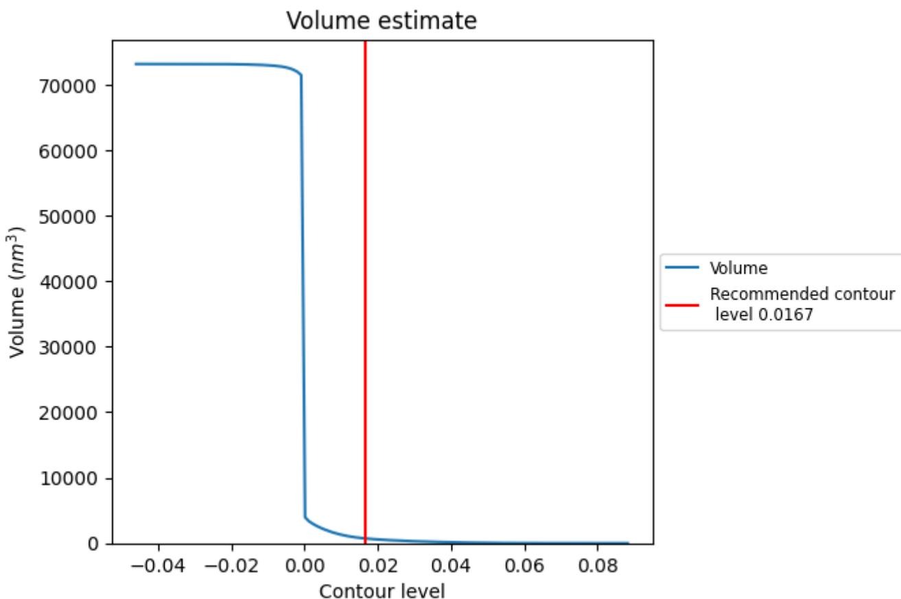
The volume at the recommended contour level is 726 nm<sup>3</sup>; this corresponds to an approximate mass of 656 kDa.
