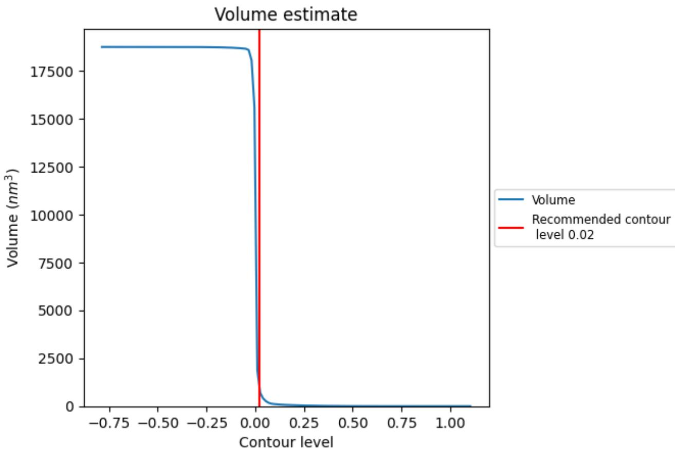
The volume at the recommended contour level is 1153 nm<sup>3</sup>; this corresponds to an approximate mass of 1041 kDa.
