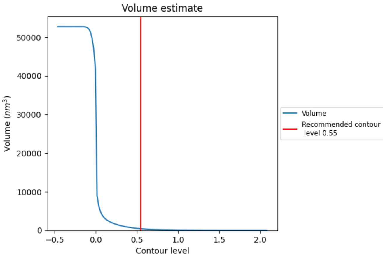
The volume at the recommended contour level is 395 nm<sup>3</sup>; this corresponds to an approximate mass of 357 kDa.
