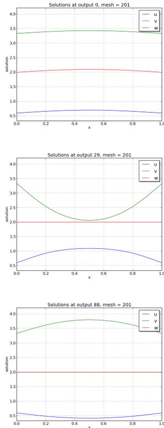
Brusselator PDE solution snapshots: left is at time  $t = 0$ , center is at time  $t = 2.9$ , right is at time  $t = 8.8$ .
