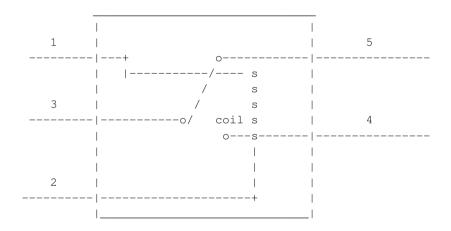
In the above diagram pin 3 is connected to pin 5, by default. By sending +12V between pin 1 and pin 2, you will will turn on a switch. Pin 1 and pin 2 will disconnect, and pin 5 and pin 4 will connect.
