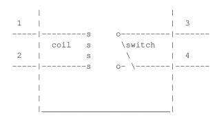
In the diagram above, pin 3 and pin 4 are disconnected by default. When you send +12V between pin 1 and pin 2, it will turn on a switch, and pin 3 and 4 are now connected.
