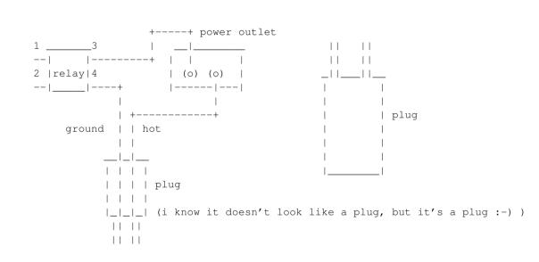
To connect the system, just connect your home electrical device to the power outlet. That is it! You don't need to make any change on the electrical device. And you can connect any kind of device to that power outlet. Plug this power outlet into any wall outlet.
