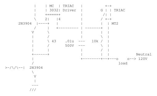
This design is for 120V. You should change resistors accordingly for 220V.
