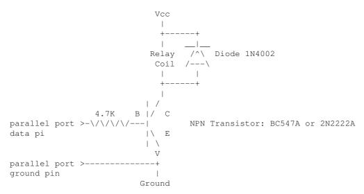
Connect Vcc with the same voltage as the relay type (usually 5 or 12V). Obviously, the relay's specifications should be scaled for your coffee-machine.
